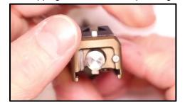
Step 20: Now you're going to put your back plate into place again. Your stainless steel striker guide is going to locate in that pocket shown below. You want to first slide that plate in just a bit, compressing the striker spring and guide down with your finger so you can capture the plate. Then using your punch, compress down on the extractor spring assembly enough to slide the back plate back in.
