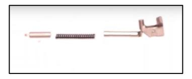
Step 12: Next you will start by compressing that striker spring, which will allow you to slide that back plate off. Be careful when releasing the striker spring, as it is under tension.
