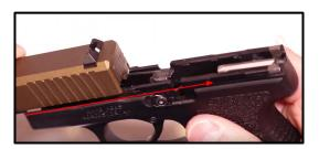
Step 23: Now line up the lug in the barrel with that hole in the frame and drop in the slide stop.
